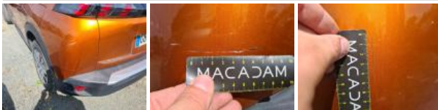
Bumper corner RL, Scratch(es), Paint
