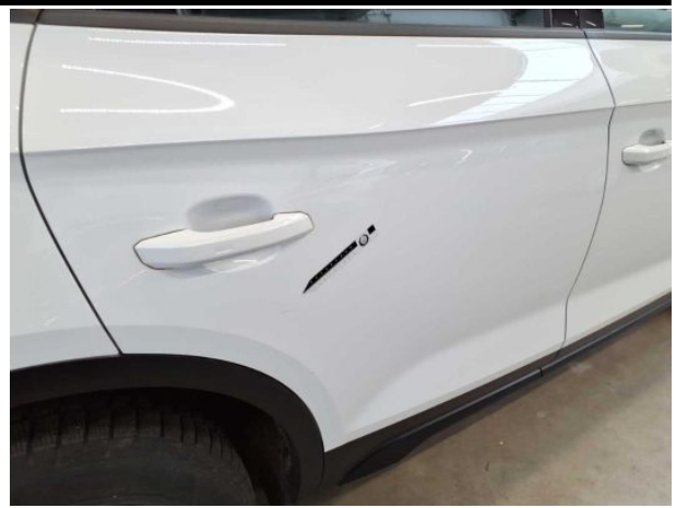
Damage #12: Door - rear right side: Door - Scratch(es) - Rep... and paint
