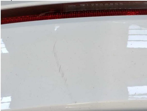
Damage #10: Rear bumper: Rear bumper - Scratch(es) - Repair and paint
