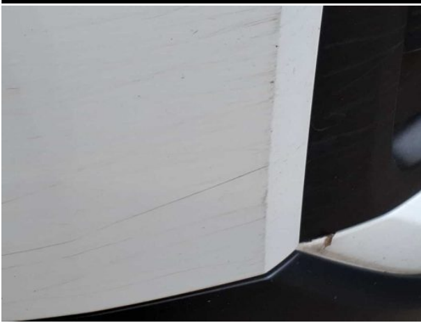
Damage #11: Front bumper: Front bumper - Scratch(es) - Repair and paint
