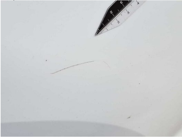
Damage #12: Door - rear right side: Door - Scratch(es) - Repair a... paint
