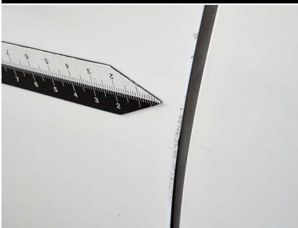
Damage #4: Door - front left side: Door edge - Scratch(es) - Smart repair
