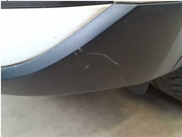
Damage #5: Front bumper: Bumper - front left side (Spoilerecke) - Scratched - Replace
