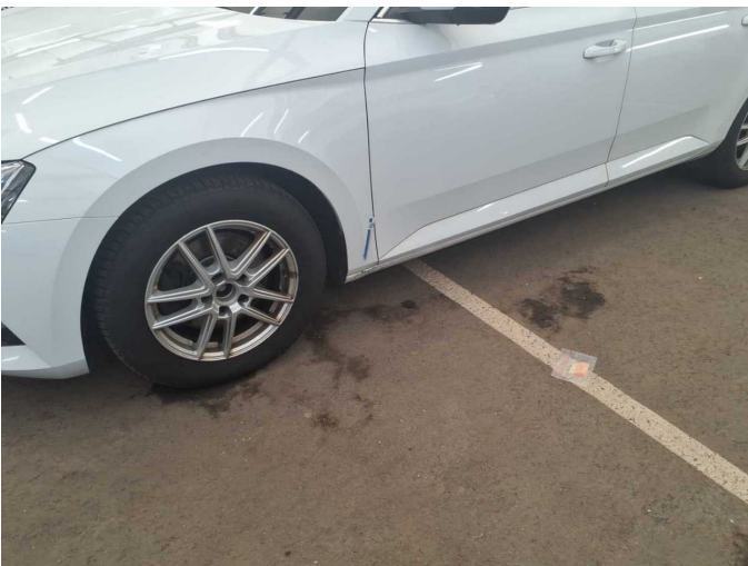
Damage 6: Sill - left side: Sill - Scratched - Repair and paint
