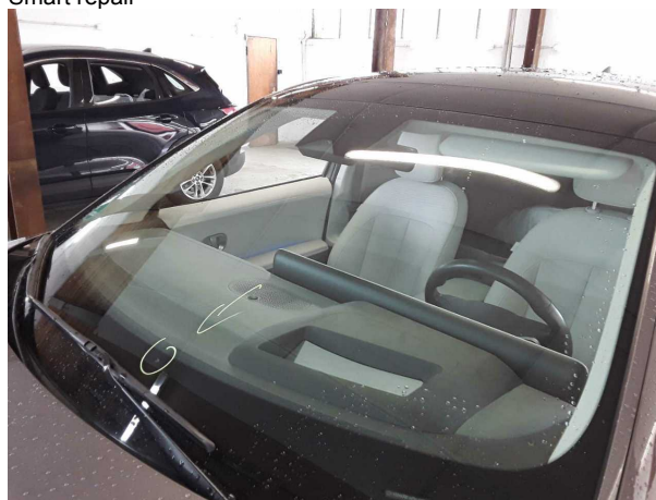
Damage #6: Vehicle glazing: Windscreen (Rissbildung) - Stone chips - Replace
