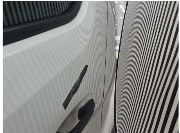
Beschädigung #3: Tür vorn links: Tür - Delle(n) - Smart Repair
