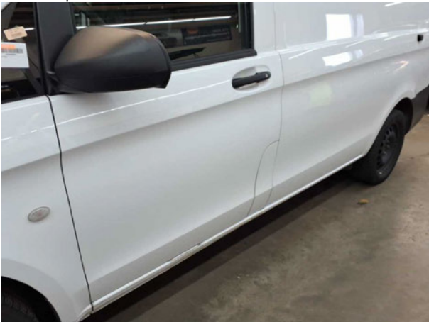
Beschädigung #3: Tür vorn links: Tür - Delle / Lackschaden - Smart Repair
