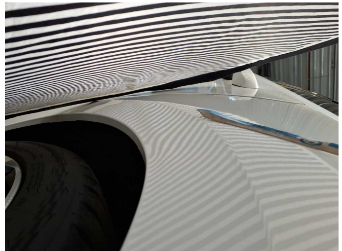
Damage 10: Side panel - rear left side: Side panel - Deformed - Repair and paint
