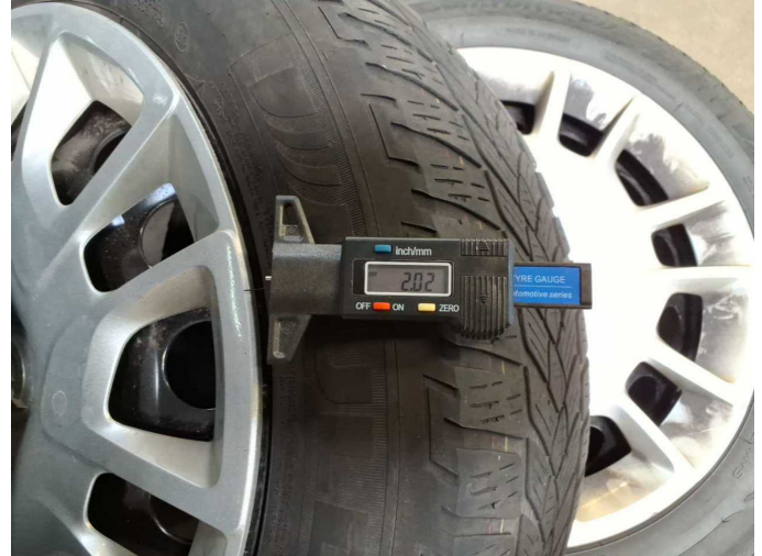
Damage 9: 2nd wheel set: 2nd wheel set (Verschließen, alle unter 3mm.) - Does not meet the leasing specifications - Replace
