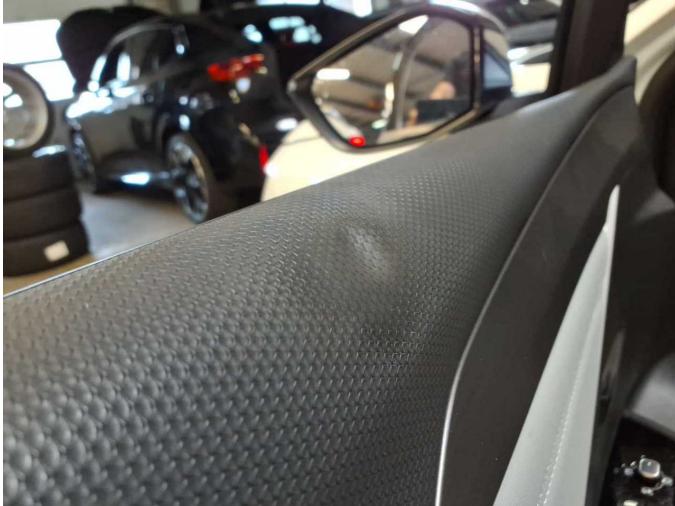
Damage 8: Trim / covers: Door trim - front left side - Deformed - Smart repair
