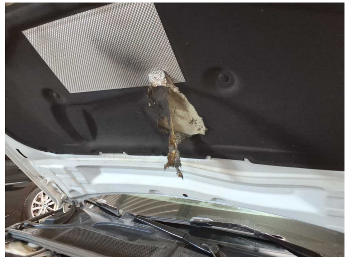
Damage 7: Bonnet: Insulation lining - Damage caused by marten / rodent - Replace
