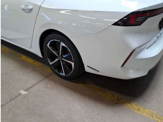
Damage 11: Rear bumper: Rear bumper - Deformed - Repair and paint
