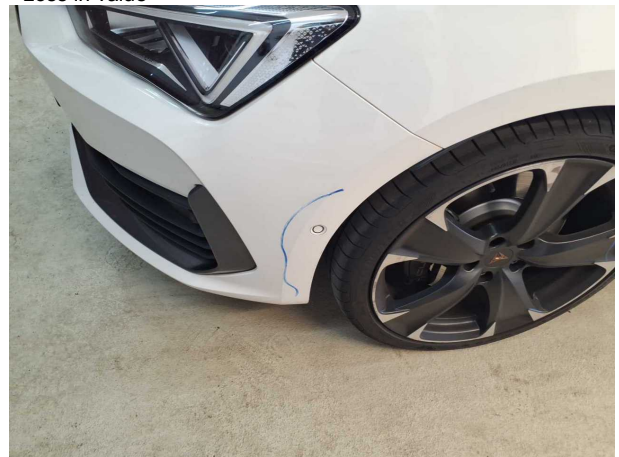
Damage #5: Front bumper: Front bumper - Scratched - Smart repair
