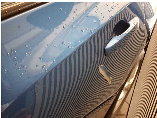
Beschädigung #4: Tür hinten links: Tür - Delle / Lackschaden - Smart Repair
