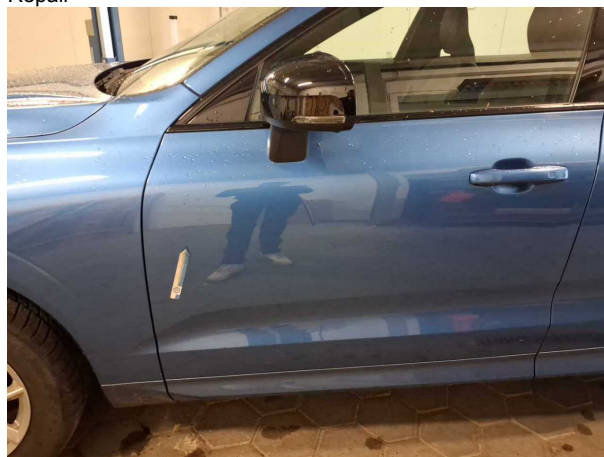
Beschädigung #6: Tür vorn links: Tür - Delle / Lackschaden - Smart Repair
