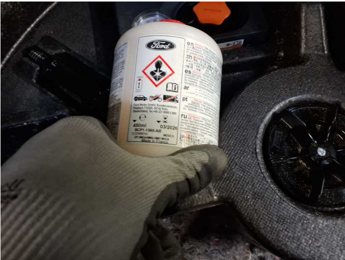
Damage 1: Equipment: Tirefit filler - Expired - Replace
