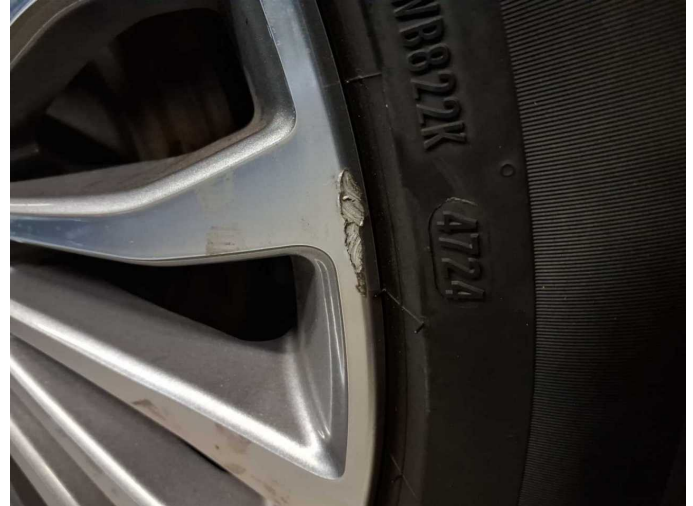
Damage 12: Wheel / tyres: Alloy rim - rear right side (Materialabtrag) - Scratched - Replace
