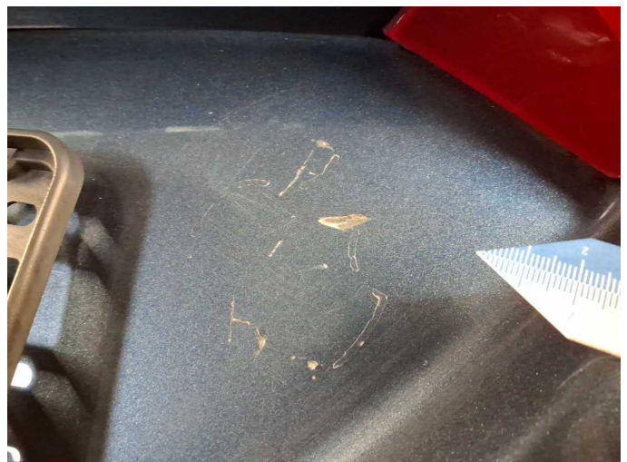
Damage 14: Boot lid / rear door: Boot lid - Scratched - Repair and paint
