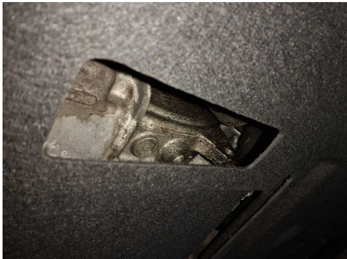
Damage 2: Gearbox: Gearbox - Leaking - Perform diagnosis
