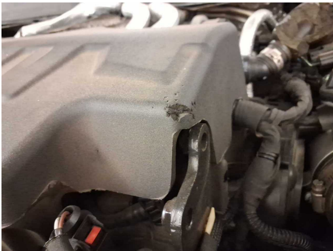
Damage 8: Engine: Engine cover - Damage caused by marten / rodent - Replace
