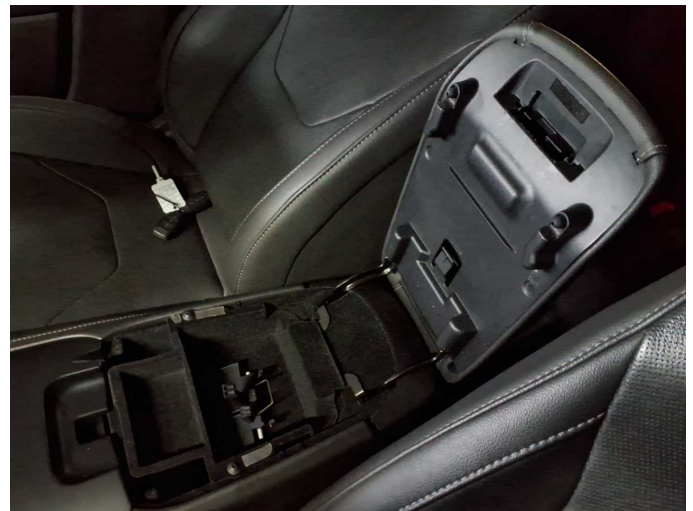
Damage 11: Seat - front: armrests - Damaged - Replace
