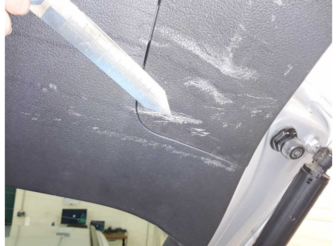
Damage 7: Boot lid / rear door: Trim - standard - lower - Scratch(es) - Replace
