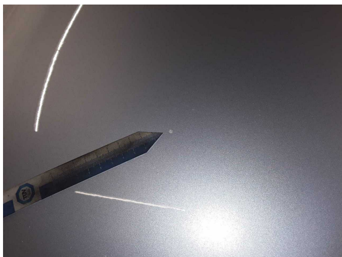
Damage 3: Bonnet: Bonnet - Stone chips - Smart repair
