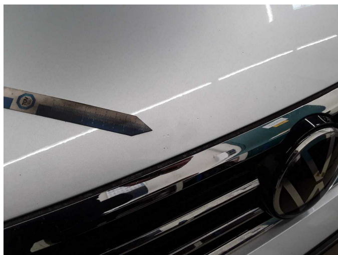
Damage 3: Bonnet: Bonnet - Stone chips - Smart repair
