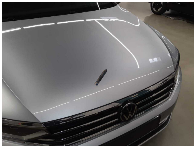
Damage 3: Bonnet: Bonnet - Stone chips - Smart repair
