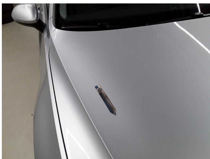
Damage 3: Bonnet: Bonnet - Stone chips - Smart repair
