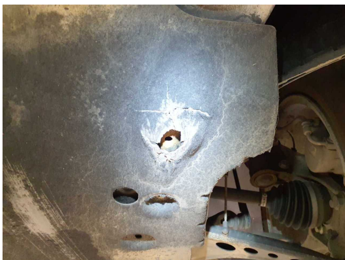
Damage 5: Body: Underbody panelling (VM) - Broken / torn - Replace
