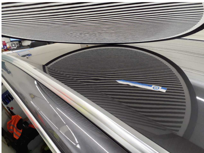
Damage 3: Roof: Roof - dent(s) - Smart repair
