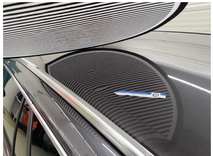
Damage 3: Roof: Roof - dent(s) - Smart repair
