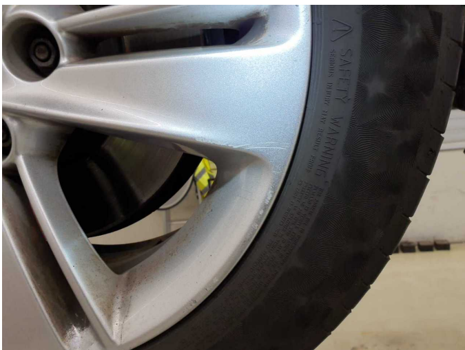
Damage 2: Wheel / tyres: Alloy rim - front left side - Scratched - Smart repair
