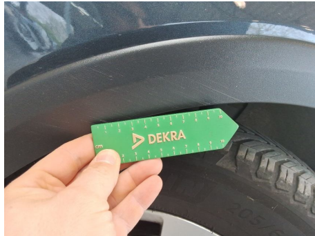
Wing extension moulding / Front Right / Scratched
