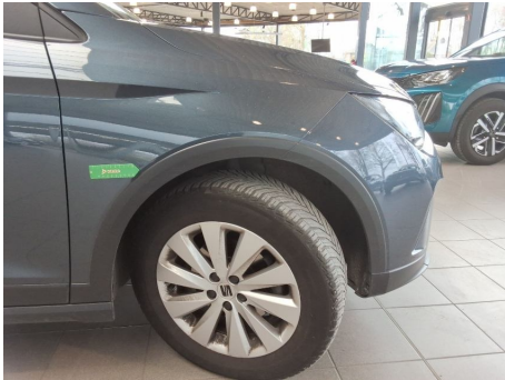
Wing extension moulding / Front Right / Scratched
