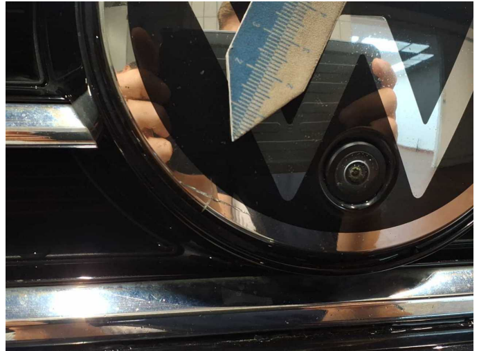
Damage 9: Front structure: Emblem - Broken / torn - Replace
