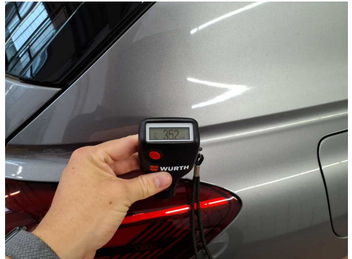
Repainting 2: Side panel - rear right side
