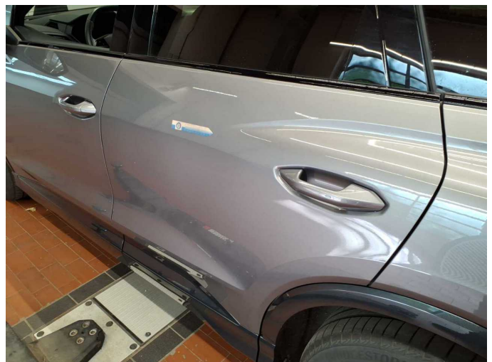
Damage 5: Door - rear left side: Door - Dent / paintcoat damage - Smart repair
