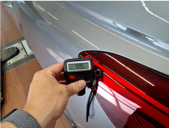
Repainting 1: Side panel - rear left side
