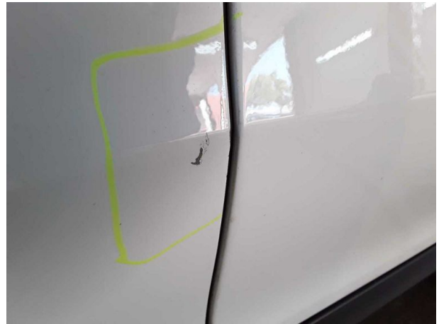
Damage #8: Door - front left side: Door - Scratched - Smart repair
