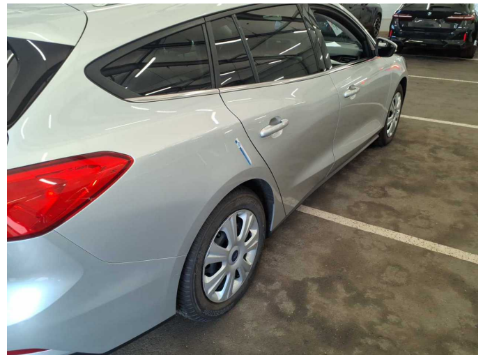
Damage 12: Side panel - rear right side: Side panel - Dent / paintcoat damage - Repair and paint
