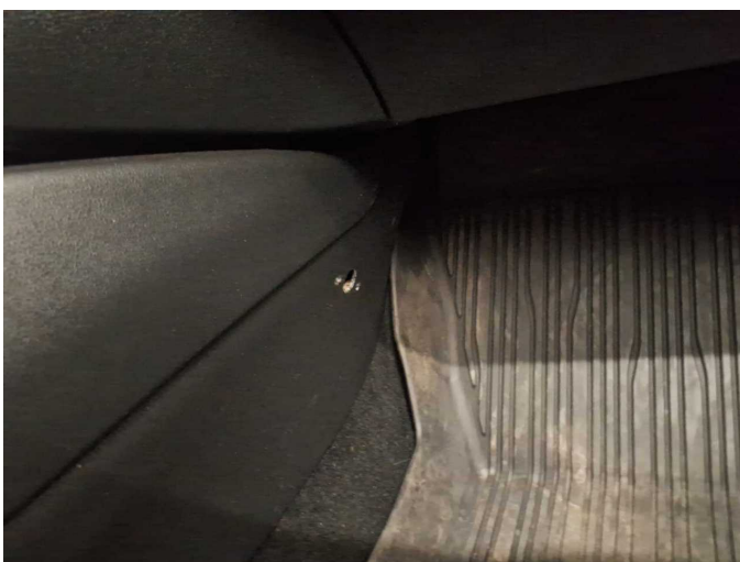
Damage 8: Instrument panel: Centre console - front (Blende rechts, Fehlbohrungen) - Differs from the original configuration - Replace
