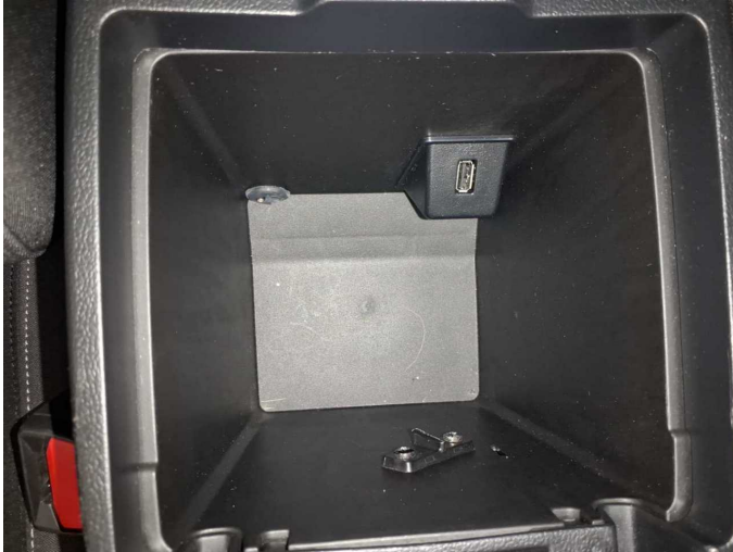
Damage 2: Interior: Arm rest, front (Deckel, Fehlbohrungen) - Differs from the original configuration - Replace
