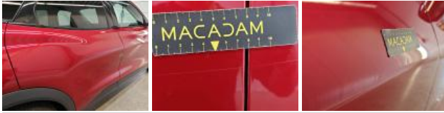
Door FR, Scratch(es), Repair and paint (complete)
