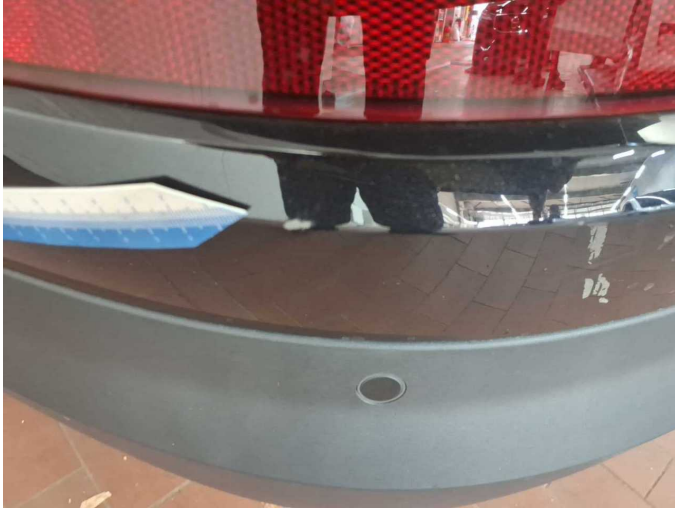
Damage 8: Rear bumper: Rear bumper - Scratch(es) - Paint
