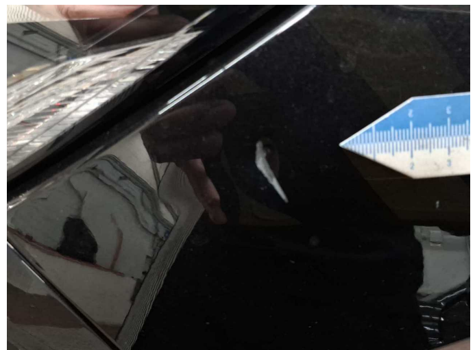
Damage 7: Mudguard - left side: Mudguard - left side - Dent / paintcoat damage - Paint
