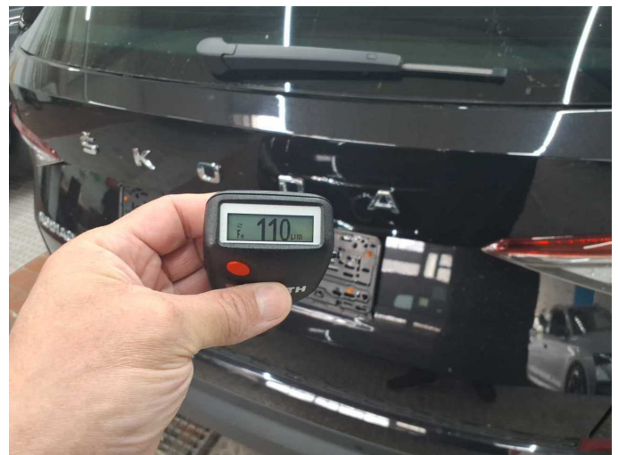
Repainting 1: Boot lid / rear door, Mudguard - right side, Bonnet, Side panel - rear right side, Door - rear right side, Door - front right side
