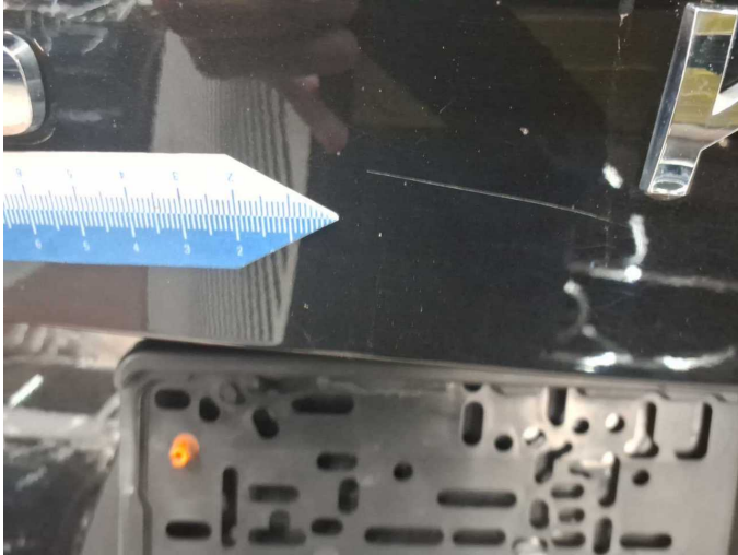
Damage 9: Boot lid / rear door: Boot lid - Dent / paintcoat damage - Paint
