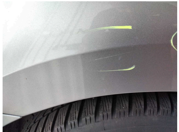
Damage 2: Side panel - rear right side: Side panel - Dent / paintcoat damage - Repair and paint
