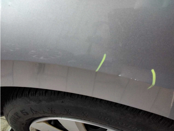
Damage 8: Side panel - rear right side: Side panel - Dent / paintcoat damage - Smart repair
