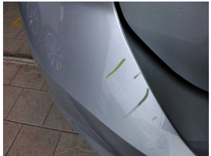
Damage 9: Rear bumper: Rear bumper - Scratch(es) - Paint
