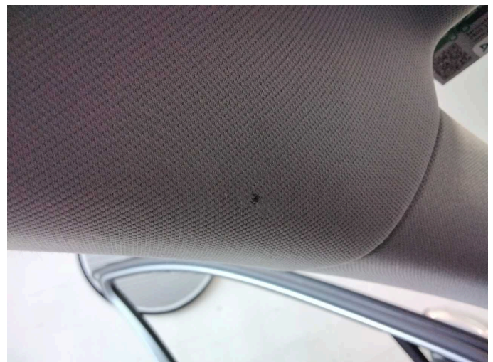
Damage 2: Trim / covers: Roof lining - Burn hole (cigarettes) - Smart repair
