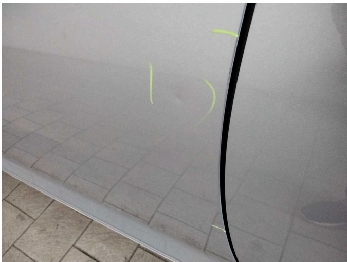
Damage 1: Door - front left side: Door - dent(s) - Smooth repair work
