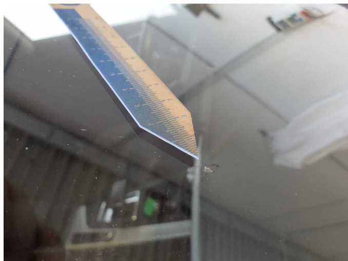
Damage 7: Vehicle glazing: Windscreen - Broken / torn - Replace
