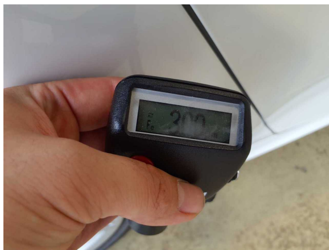
Repainting 2: Side panel - rear right side
