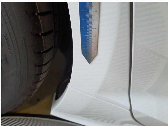
Damage 5: Side panel - rear right side: Side panel (Wellig) - Unprofessionally repaired - Repair and paint
