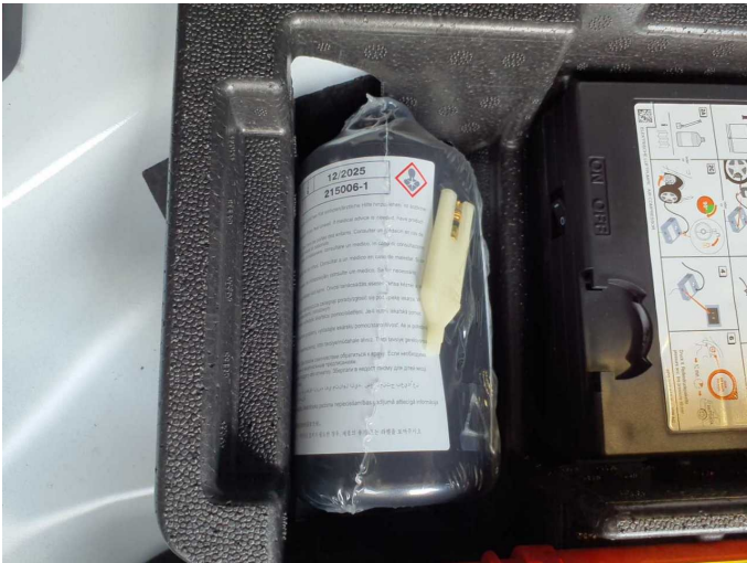
Damage 2: Equipment: Tirefit filler - Expired - Replace
