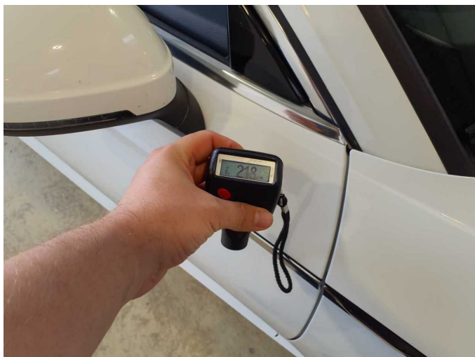
Repainting 1: Roof rail - right side, Mudguard - right side, Door - rear right side, Door - front right side
