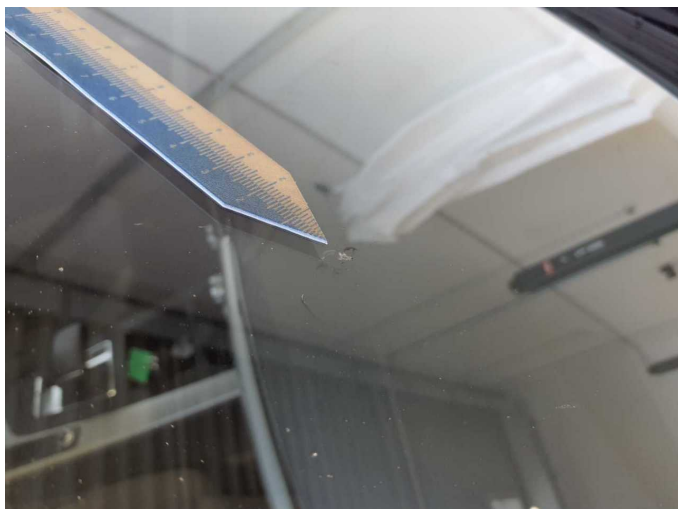
Damage 7: Vehicle glazing: Windscreen - Broken / torn - Replace
