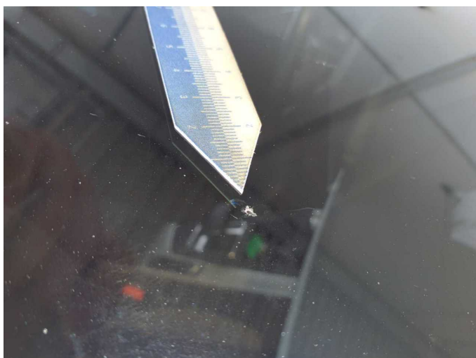
Damage 7: Vehicle glazing: Windscreen - Broken / torn - Replace
