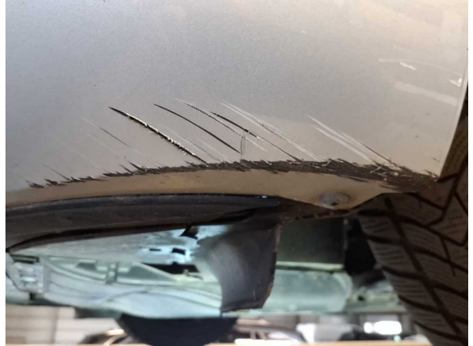
Damage 6: Front bumper: Front bumper - Scratched - Paint
