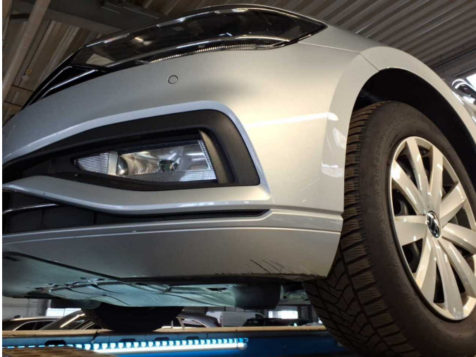
Damage 6: Front bumper: Front bumper - Scratched - Paint
