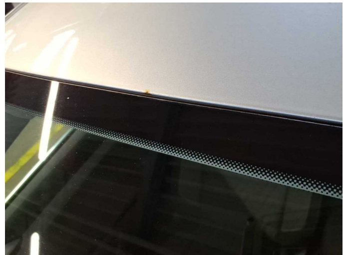
Damage 4: Roof: Roof - Corrosion - Smart repair
