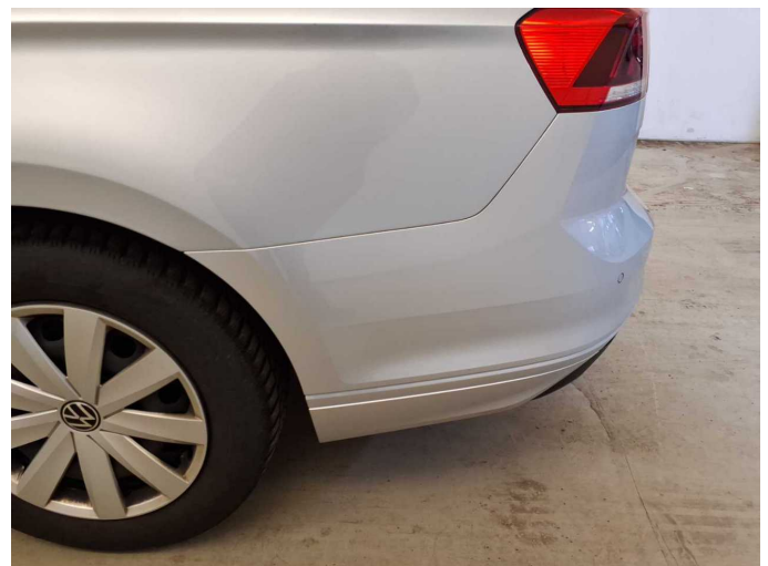
Damage 5: Rear bumper: Rear bumper (Farb unterschied) - Unprofessionally repaired - Paint
