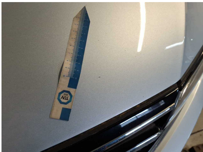
Damage 7: Bonnet: Bonnet - Stone chips - Paint
