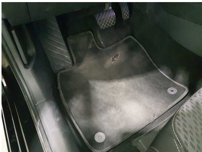
Wear and tear 1: Trim / covers: Floor mats - Broken / torn - Replace
