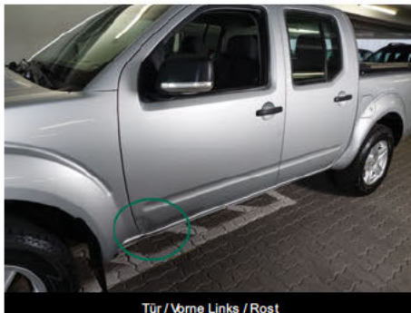
Tür / Vorne Links / Rost
