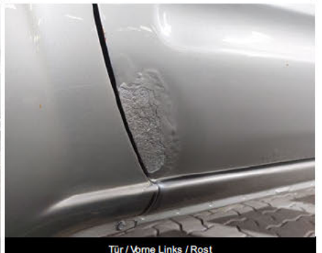
Tür / Vorne Links / Rost
