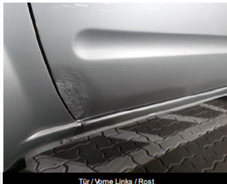
Tür / Vorne Links / Rost
