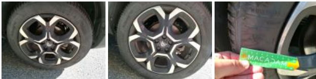
Tyre RR, Out of tolerance, Replace
