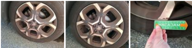
Tyre RL, Out of tolerance, Replace
