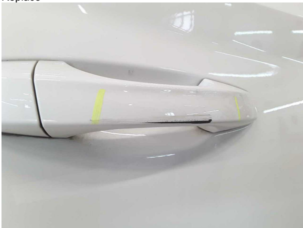
Damage #3: Door - rear right side: Door handle - outside - Scratched - Smart repair
