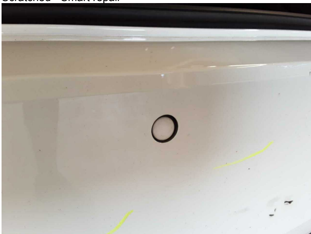
Damage #4: Rear bumper: Parking sensors - centre - Loose - Un- / install
