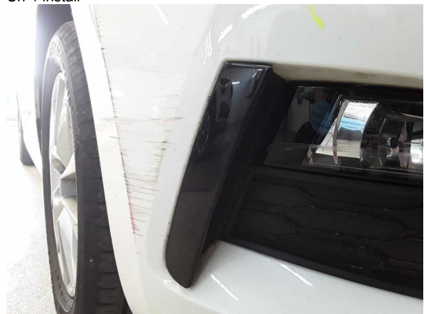
Damage #5: Front bumper: Spoiler - Damaged - Replace
