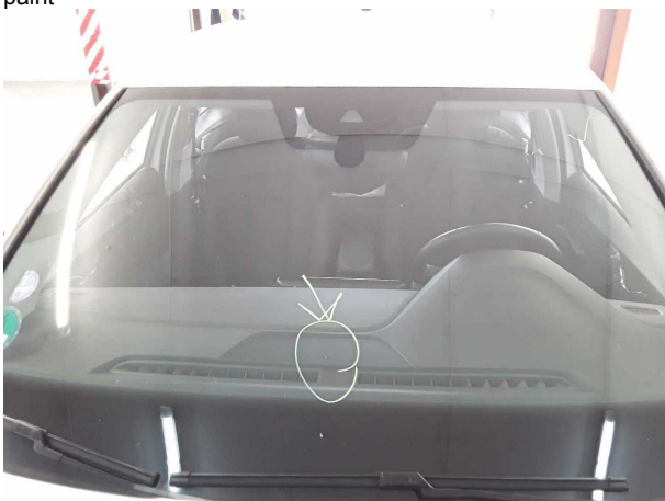
Damage #7: Vehicle glazing: Windscreen (Rissbildung) - Stone chips - Replace
