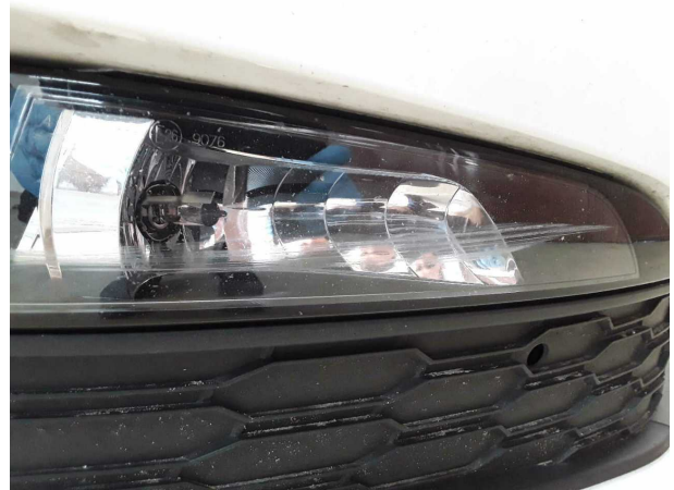
Damage #2: Fog lamp: Fog lamp - front right side - Scratched - Replace
