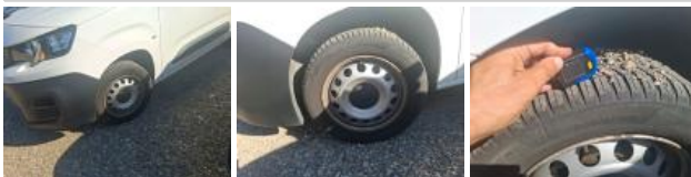
Tyre RL, Out of tolerance, Replace
