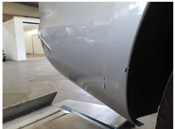
Damage 7: Rear bumper: Rear bumper - Scratch(es) - Paint
