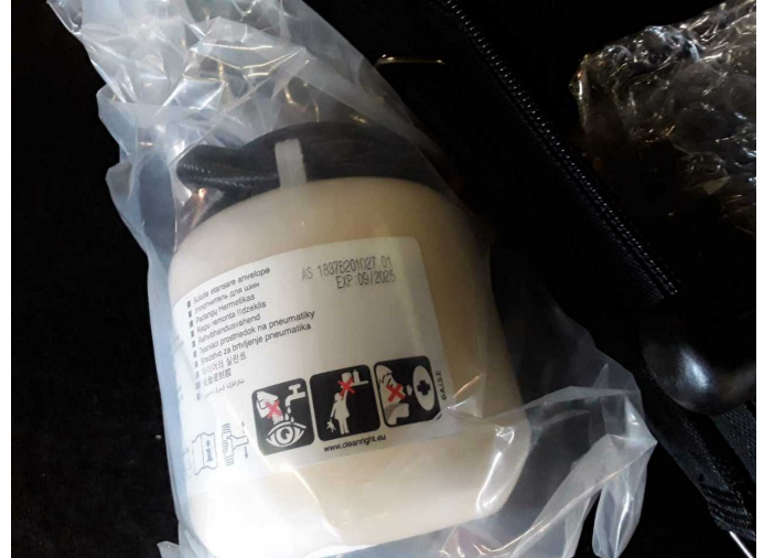
Damage 2: Equipment: Tirefit filler - Expired - Replace
