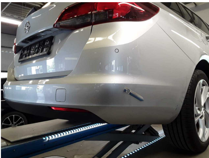
Damage 7: Rear bumper: Rear bumper - Scratch(es) - Paint
