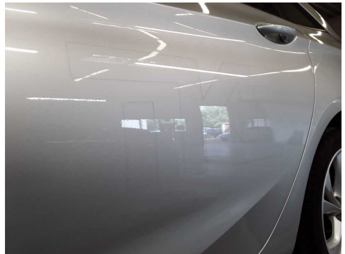
Damage 6: Body: Body (Klebereste) - Glued / labelled - De-glug / neutralise
