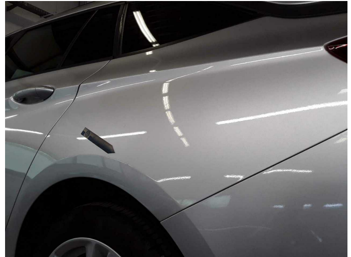
Damage 8: Side panel - rear left side: Side panel - Dent / paintcoat damage - Repair and paint
