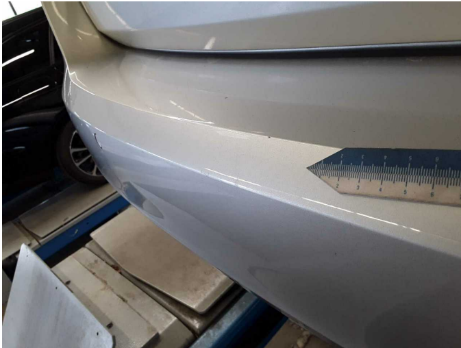
Damage 7: Rear bumper: Rear bumper - Scratch(es) - Paint
