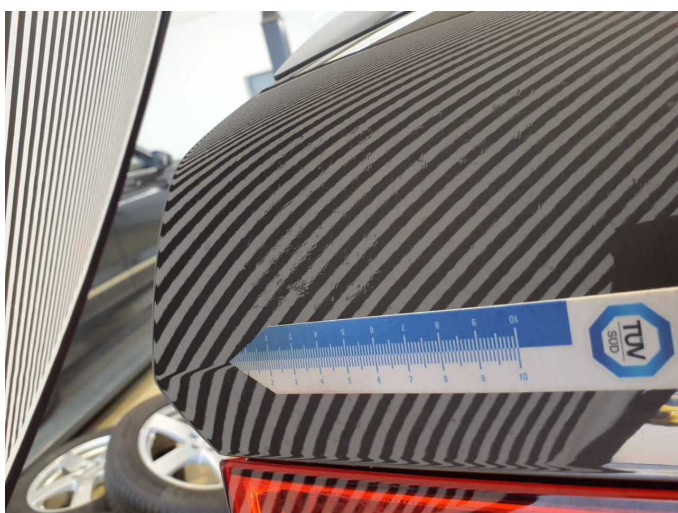
Damage 13: Boot lid / rear door: Boot lid (Spachtelmasse eingefallen) - Unprofessionally repaired - Repair and paint
