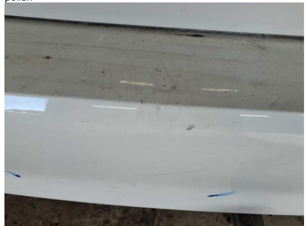
Damage #2: Rear bumper: Rear bumper - Scratch(es) - Cove... polish
