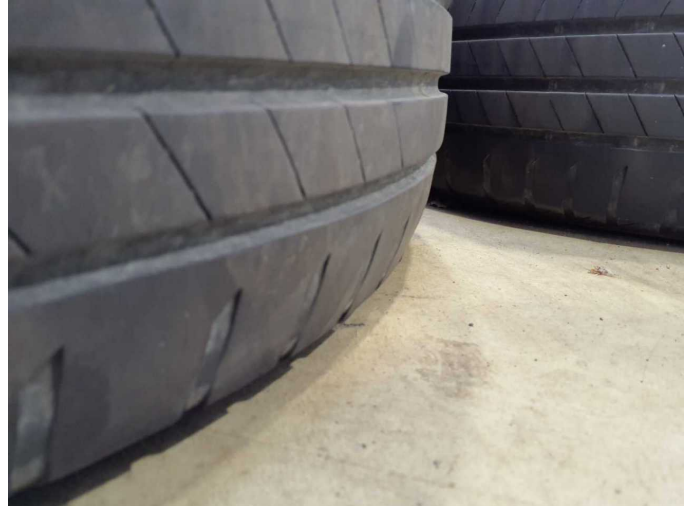
Damage 8: 2nd wheel set: Tyres - complete set - Worn - Replace
