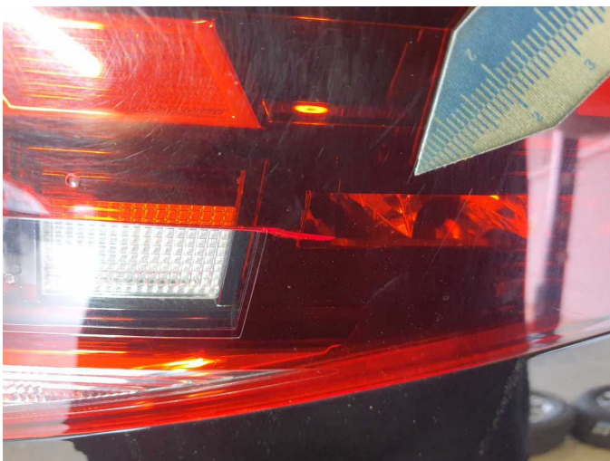
Damage 7: Tail light: Tail lamp - left side - Broken / torn - Replace
