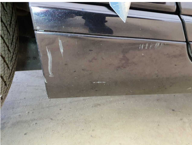
Damage 9: Sill - right side: Trim - Scratch(es) - Paint
