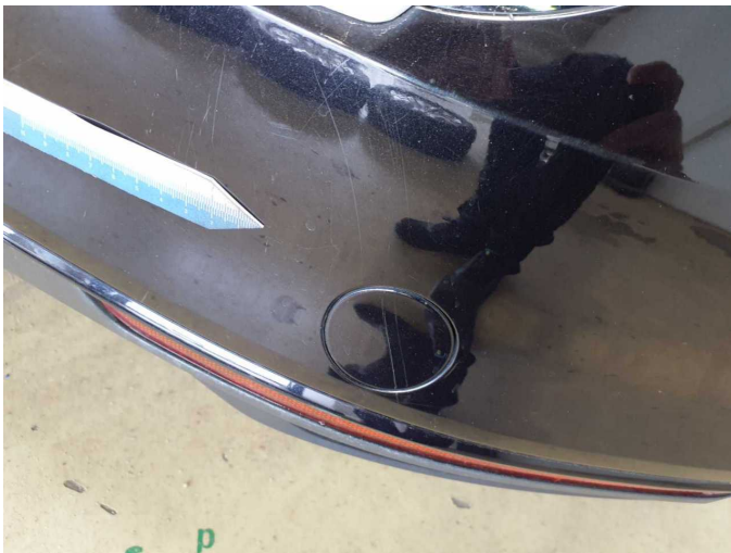
Damage 12: Rear bumper: Rear bumper - Dent / paintcoat damage - Repair and paint
