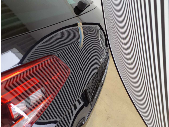
Damage 13: Boot lid / rear door: Boot lid - Dent / paintcoat damage - Repair and paint
