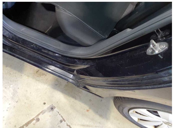
Damage 2: Side panel - rear left side: Sill - Scratch(es) - Smart repair
