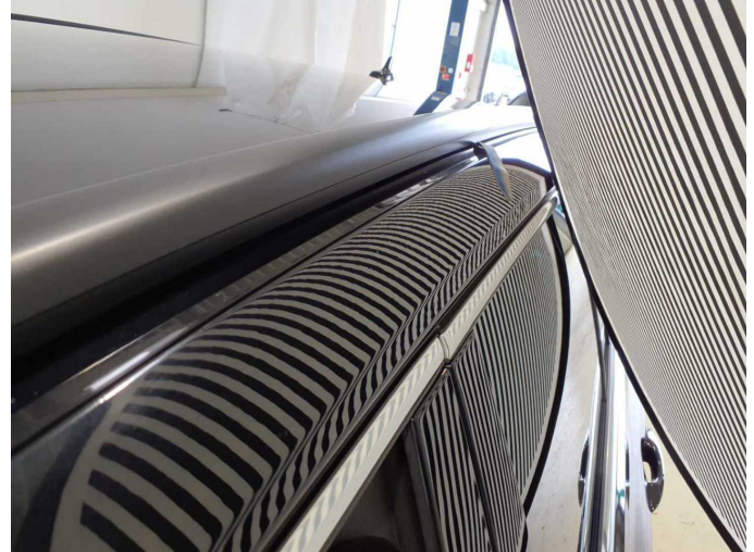
Damage 10: Roof: Roof rail - left side (Einschlüss und wellig) - Paint defect - Repair and paint
