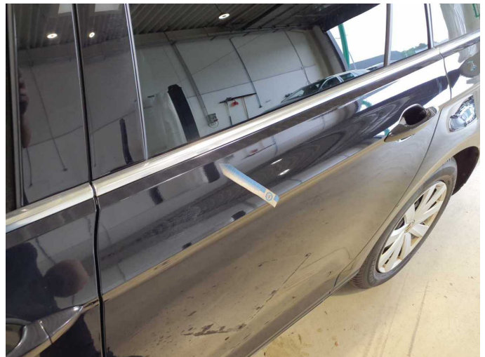
Damage 4: Door - rear left side: Door (Sprü nebel) - Paint defect - Smart repair
