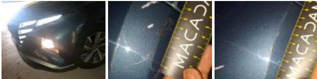
Door RR, Dent(s), Repair and paint (complete)
