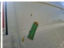
Boot door panel RR, Dent(s), Repair and paint (complete)
