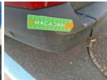
Bumper R, Deformed / Strained, Replace
