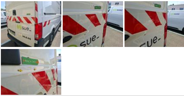
Bumper corner RR, Deformed / Strained, Replace
