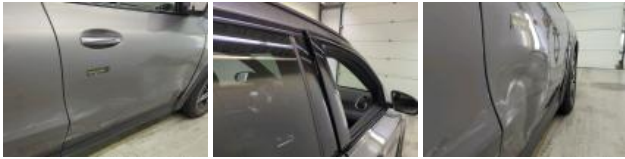
Door FR, Deformed / Strained, Replace and paint
