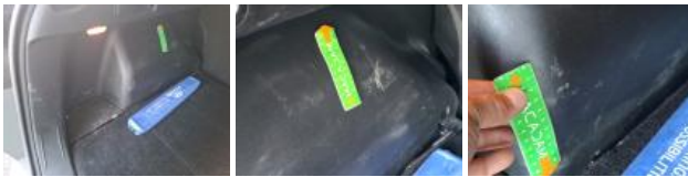
Internal boot lining R, Scratch(es), Replace
