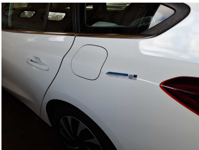
Damage 2: Side panel - rear left side: Side panel (Klarlackmangel) - Paint defect - Smart repair
