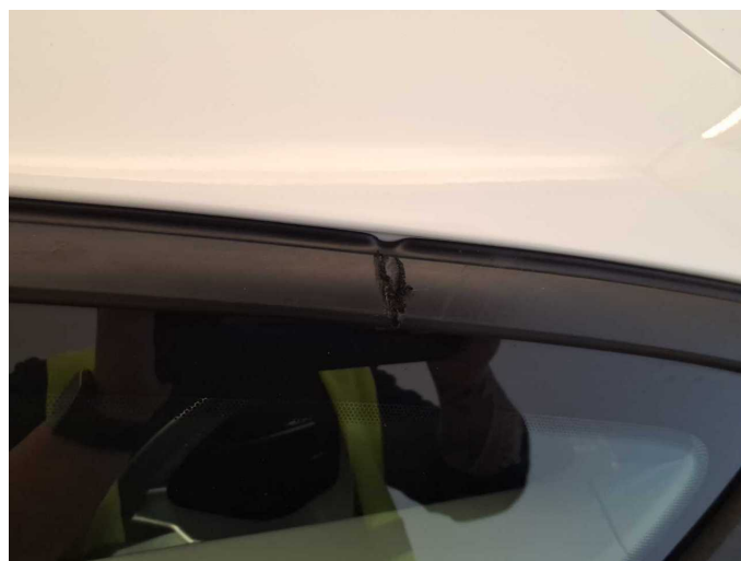
Damage 3: Vehicle glazing: Triangular window - left side (Dichtung) - Broken / torn - Replace
