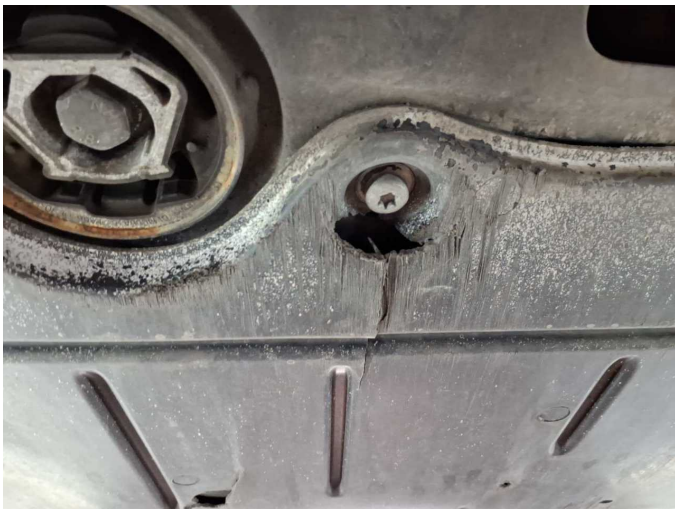
Damage 5: Body: Underbody panelling - Damaged - Replace
