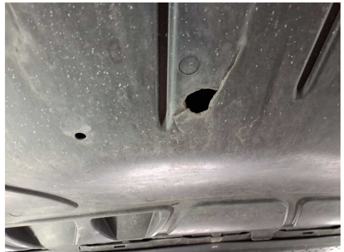
Damage 5: Body: Underbody panelling - Damaged - Replace
