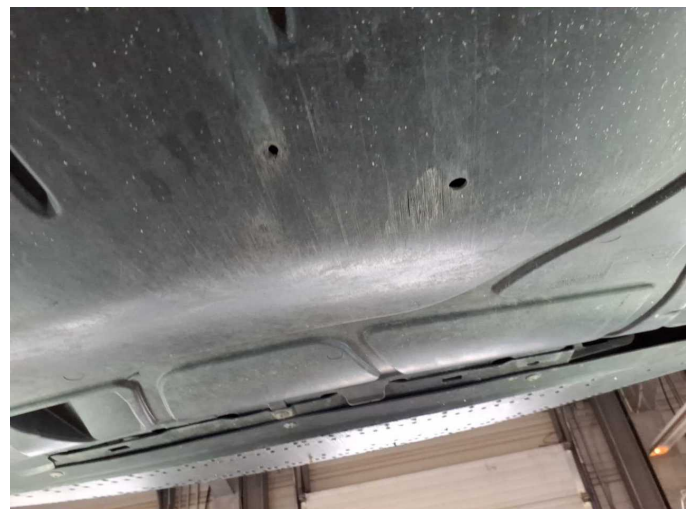
Damage 5: Body: Underbody panelling - Damaged - Replace
