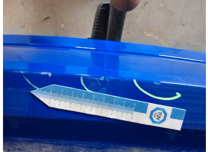
Damage 9: Rear bumper: Rear bumper - Scratch(es) - Paint
