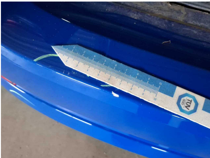
Damage 9: Rear bumper: Rear bumper - Scratch(es) - Paint
