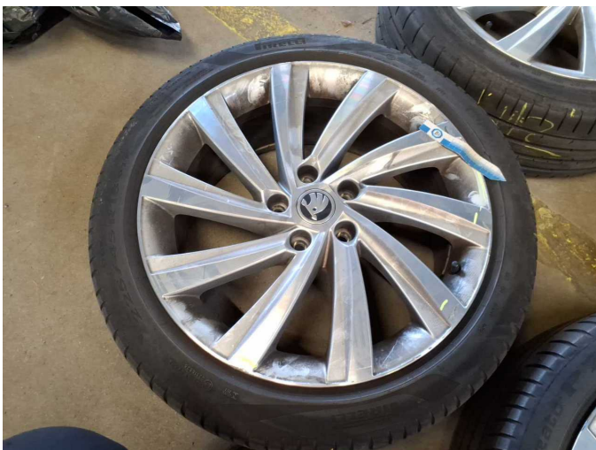
Damage 4: 2nd wheel set: 1 tyre - Damaged - Replace
