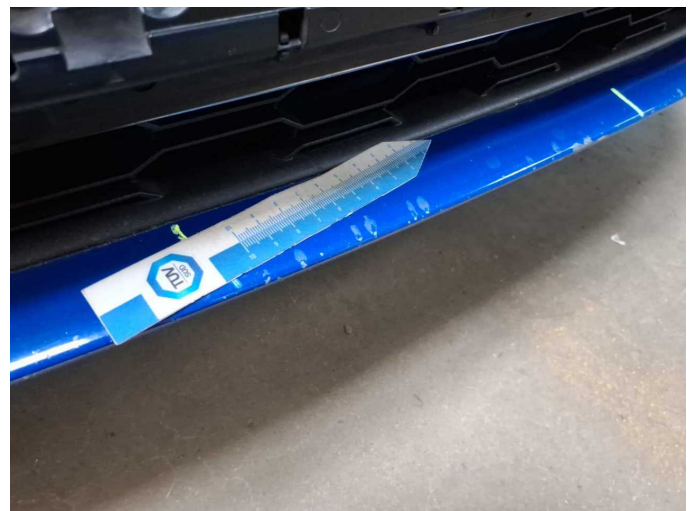
Damage 11: Front bumper: Front bumper - Scratched - Repair and paint
