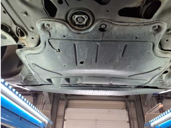
Damage 5: Body: Underbody panelling - Damaged - Replace
