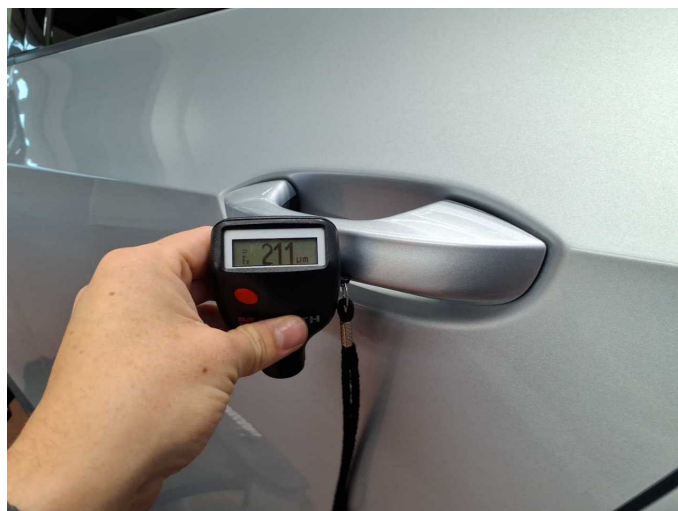
Repainting 2: Door - rear left side
