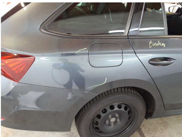
Damage #8: Side panel - rear right side: Side panel - Deformed - Repair and paint
