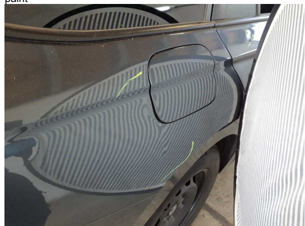
Damage #8: Side panel - rear right side: Side panel - Deform... - Repair and paint
