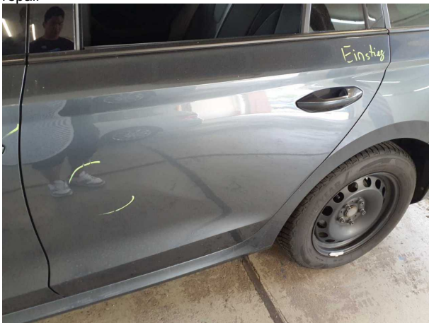
Damage #7: Door - rear left side: Door - dent(s) - Repair and paint
