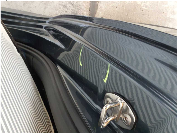
Damage #3: Side panel - rear right side: Sill - dent(s) - Smart repair
