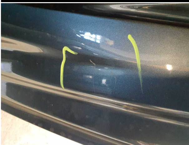
Damage #4: Side panel - rear left side: Sill - Scratched - Smart repair
