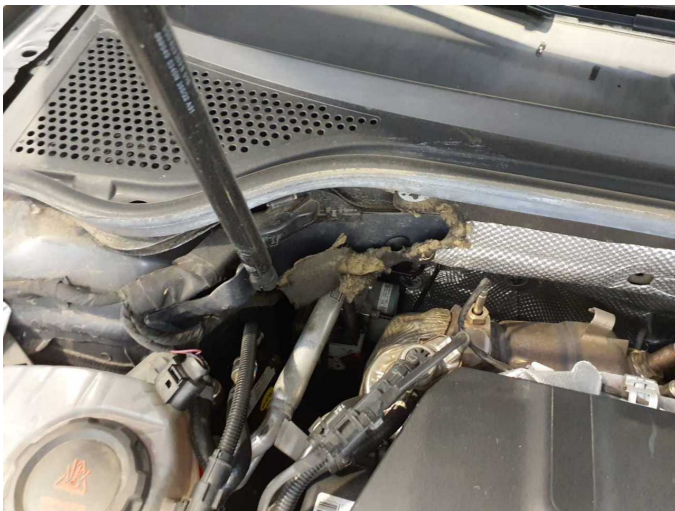
Damage 6: Cab: Insulation lining - Damage caused by marten / rodent - Replace
