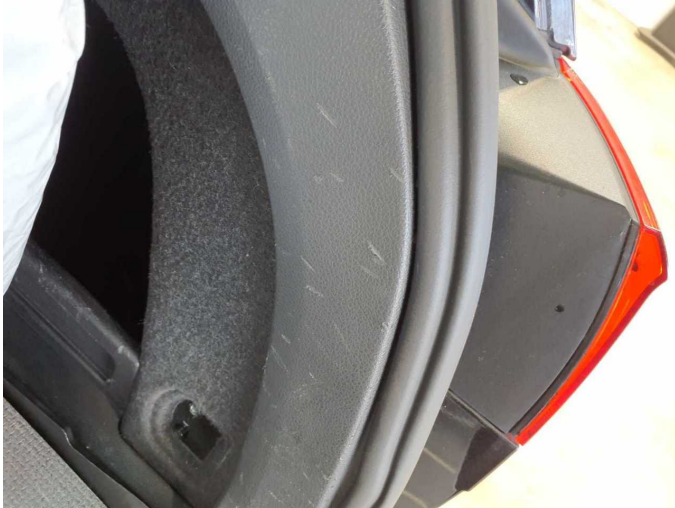
Damage 8: Trim / covers: Boot lining - Scratch(es) - Loss in value
