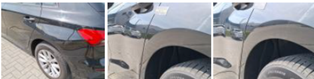
Door RL, Repaired, Acceptable
