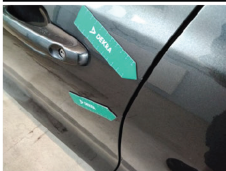
Tür / Vorne Links / Kratzer
