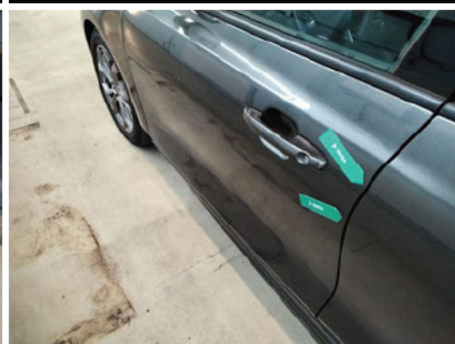
Tür / Vorne Links / Kratzer
