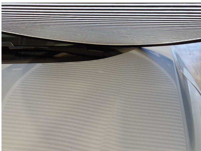
Damage 6: Body: Body (Mehrkosten möglich) - Damage by hail - repair according to calculation
