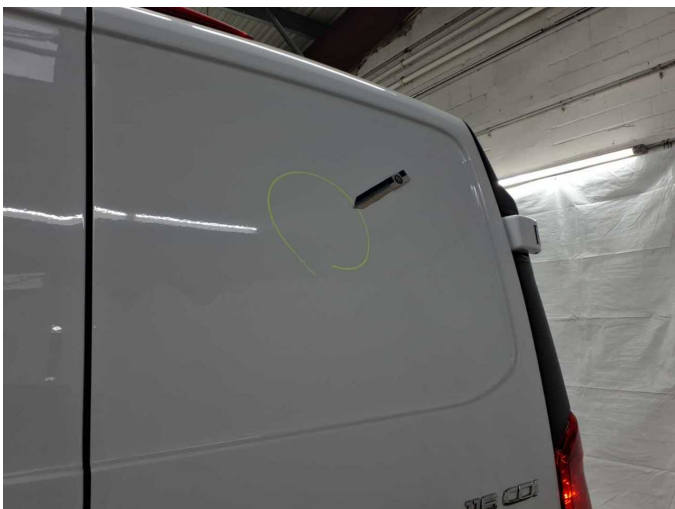
Damage 3: Boot lid / rear door: Rear door - right side - dent(s) - Smooth repair work
