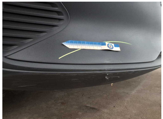
Damage 10: Front bumper: Front bumper - Scratched - Replace
