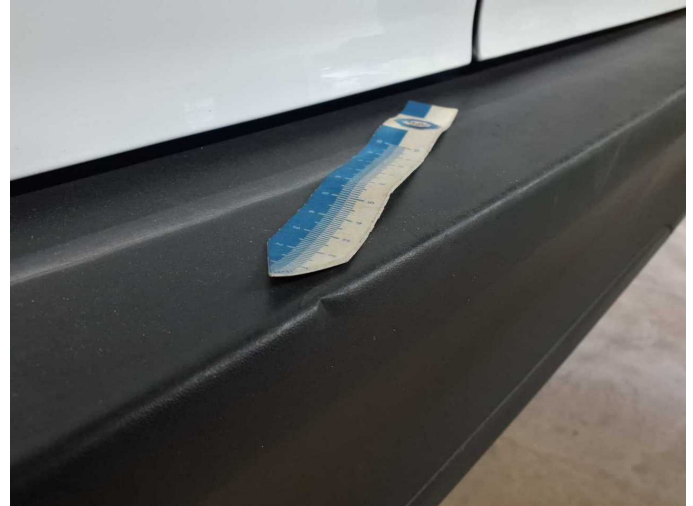
Damage 7: Rear bumper: Rear bumper - Dent / paintcoat damage - Loss in value
