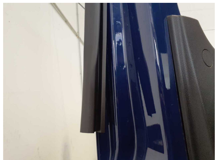
Damage 1: Door - front left side: Door seal - Loose - Un- / install
