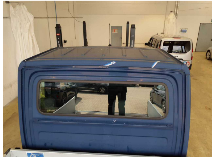
Damage 4: Roof: Roof (Dachkante) - Corrosion - Smart repair
