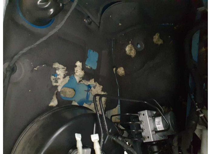
Damage 8: Cab: Insulation lining - Damage caused by marten / rodent - Replace
