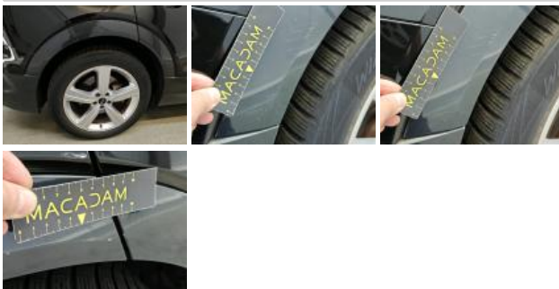
Wheel arch cover FR, Scratch(es), Replace
