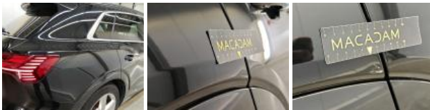
Wheel arch cover RR, Scratch(es), Replace
