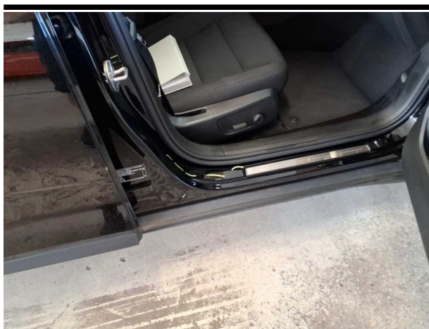
Damage #3: Sill - right side: Sill - Scratch(es) - Cover / polish
