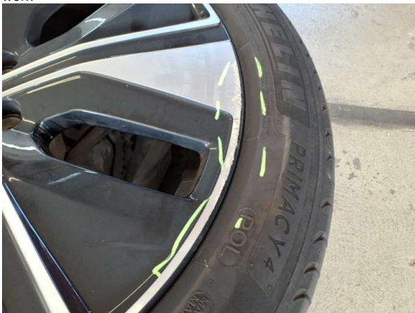
Damage #10: 2nd wheel set: 2 alloy rims - Scratched - Loss in value
