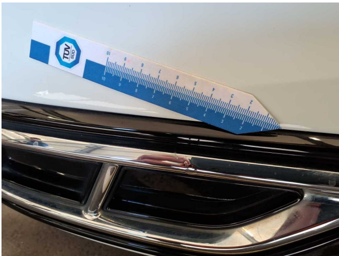
Damage 5: Rear bumper: Spoiler - Deformed - Loss in value
