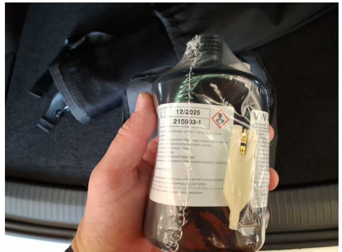
Damage 1: Equipment: Tirefit filler - Expired - Replace
