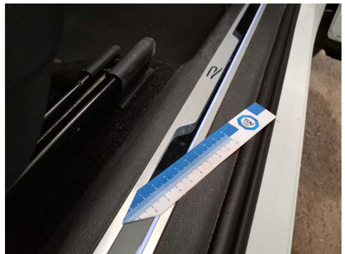
Wear and tear 1: Trim / covers: Sill - front right side - dent(s) - No deduction
