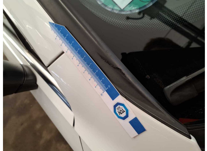
Damage 3: Roof: Cowl - right side - Scratched - Replace
