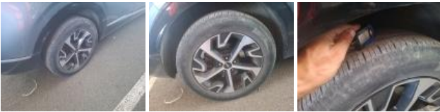
Tyre RL, Out of tolerance, Replace
